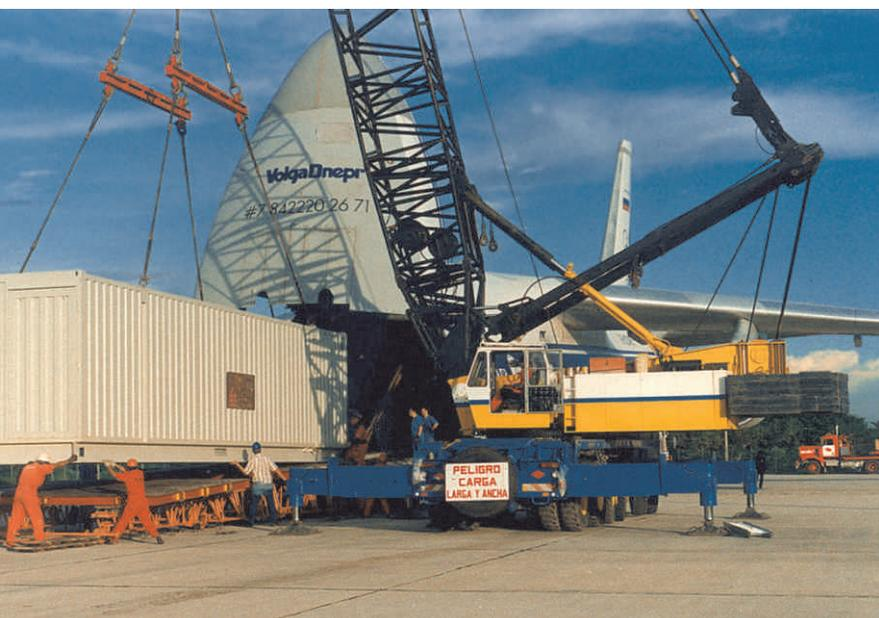
■ January 2004: Volga-Dnepr carried an 82 tonnes stainless steel vessel with foal glass lining for an oil and gas customer from Calgary in Canada to Pittsburg, USA. The most specific feature of this operation was the size of the vessel; more than 17 meters long, 3.3m wide and 3.5m high.
